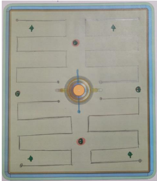
Figure 12. Sketch proposal 2: implemented cooling circuit.
