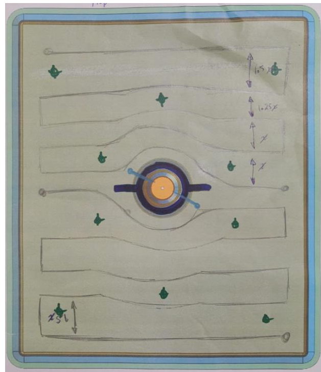
Figure 11. Sketch proposal 1: two parts, two milled channels.
