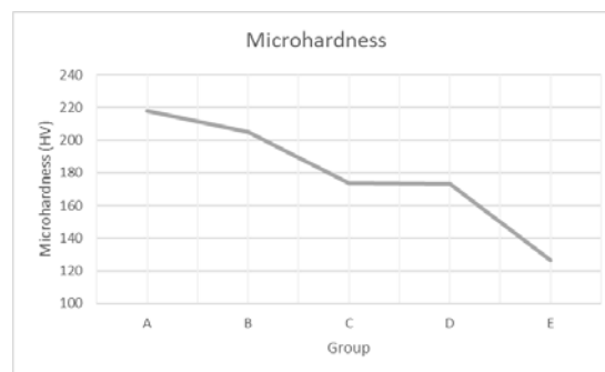
Figure 5. Evolution of the microhardness as a function of the sub-critical annealing temperature.
