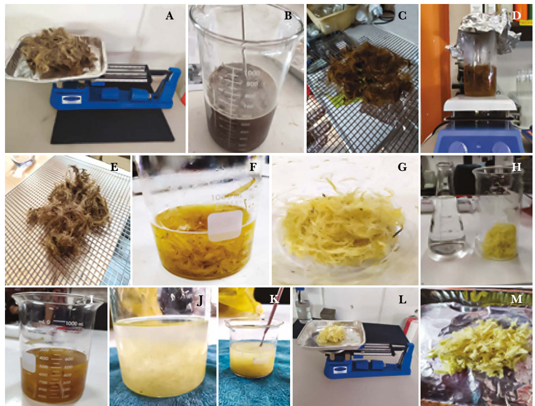
Figure 2. Cellulose extraction process from oil palm bagasse. A: Bagasse weighing; B: Pre-treatment; C: Drying in conventional furnace; D: Acid hydrolysis; E: Drying; F: Chlorination; G: Drying; H-I: Alkaline extraction; J: Blanching; K: Rest; L: Dry fiber/weighing; M: Cellulose.
