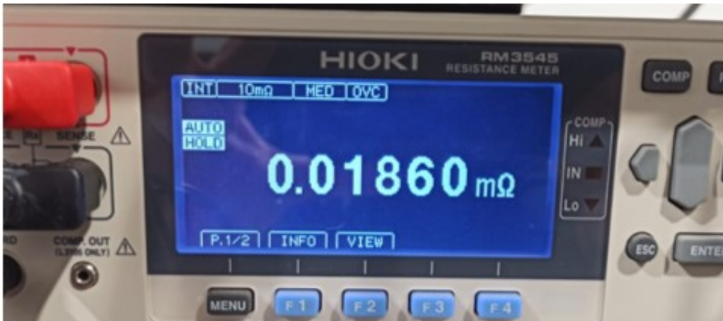
Figure 13: Milometer showing the measurement on a copper busbar
