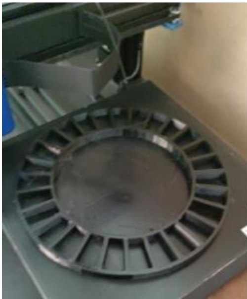
Figure 2. 3D-printed packaging insert final result achieved using the parameters configured on the equipment for manufacturing the part.
