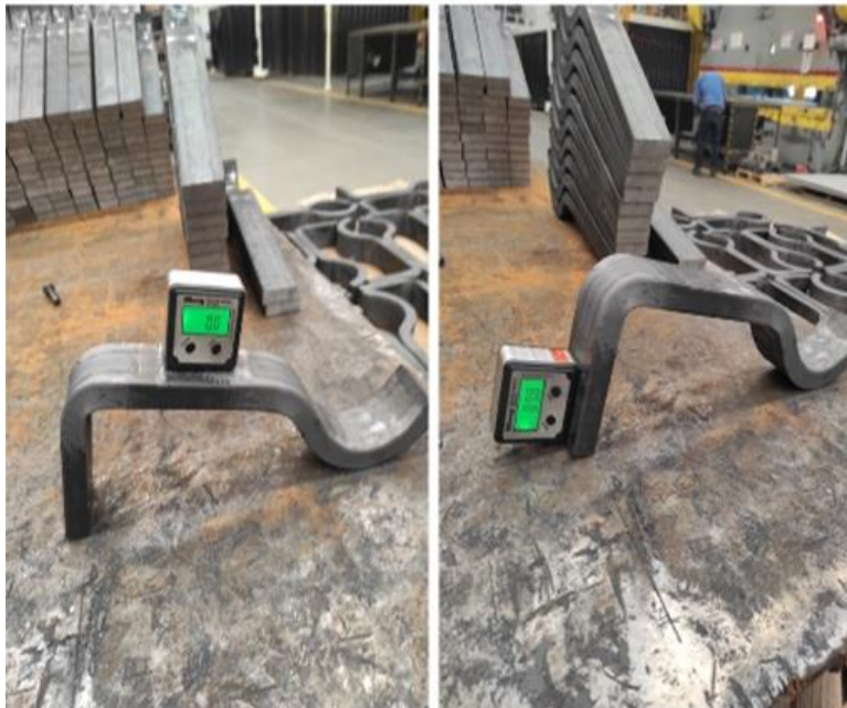
Figure 4. Angle measurements in pieces subjected to the bending process.
