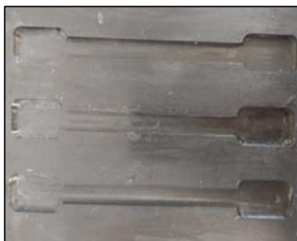
Figure 3: Molds used for the production of composites.
