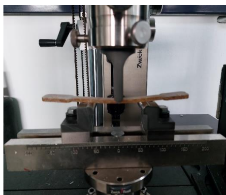
Figure 4: Flexural testing of composite materials.
