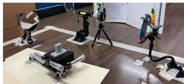
Figure 8 Final Schlieren system Source: Own Elaboration
